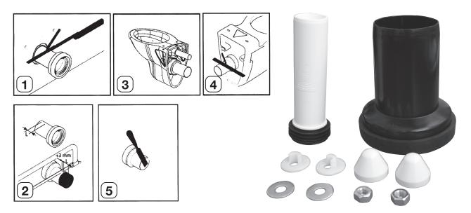
Picture (1 and 2) Install clean water and sewage extension pipes in the wall and let it fully seated. Pull a line on the pipe putting a scale to surface of the wall.
